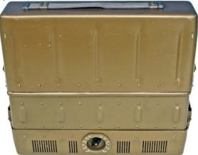
Enclosure of R-353L version A. Note the AC mains voltage selector in a round recess of the clip-on mains power unit. A separate accumulator pack of almost similar dimensions could be fitted in place of the mains power unit.
