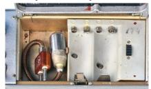
Stored data was saved in the memory, powered by two back-up batteries which were located under a hinged panel on the transmitter unit along with an operator's lamp.
